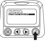
18. Once the "Use Defaults", "Custom Setup" and "Automatic Scan" functions have been set touch the "Menu Button" to return to the main menu.
